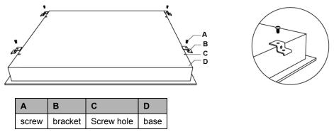
Adjust the bracket position to suit for different work surface's thickness.
